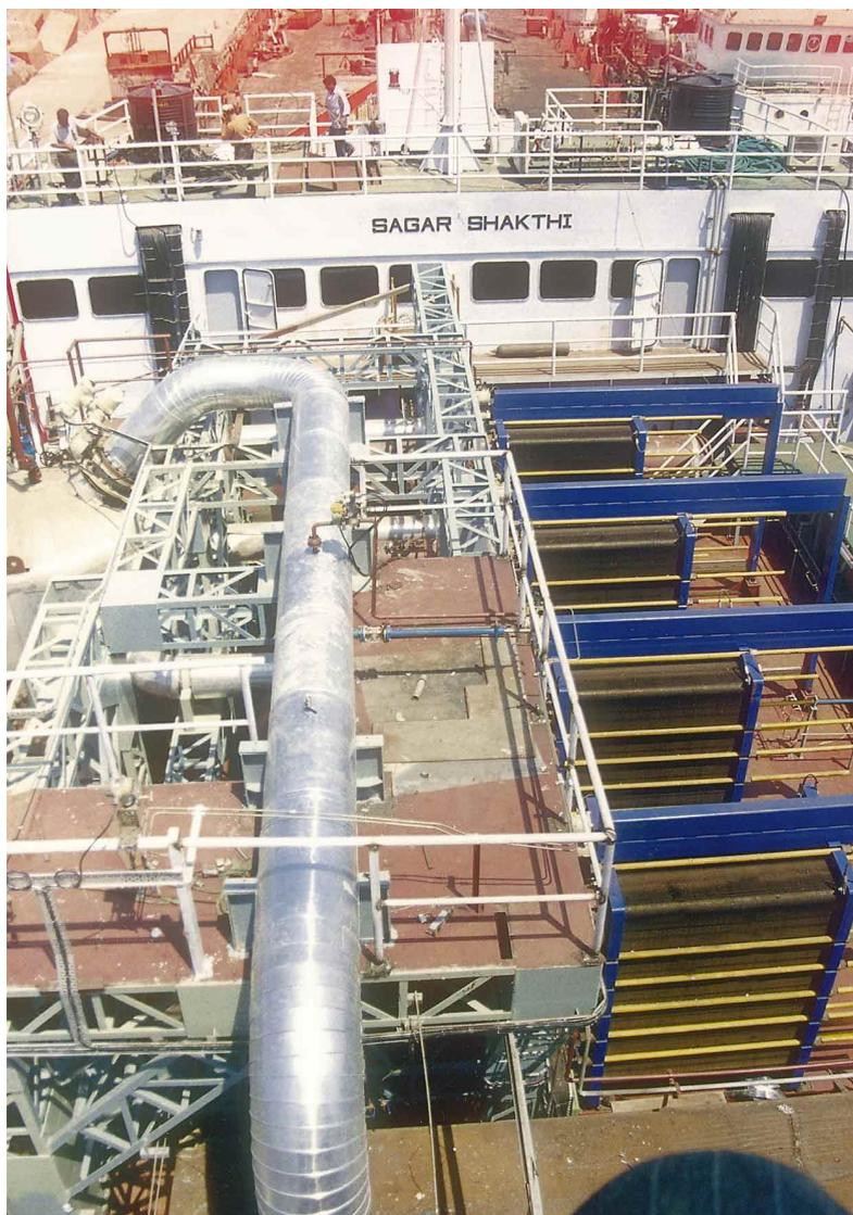
*A view of components of OTEC plant assembled on board Sagar Shakthi.*
