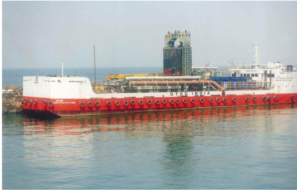
*OTEC barge Sagar Shakti constructed by NIOT with all installations for IMW OTEC power generation.*
