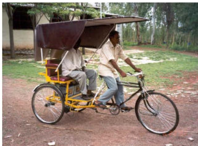
Figure 2. Motor-assisted pedal cycle rickshaw.
