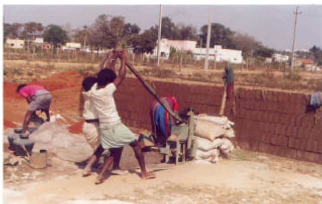
Figure 6. Production stabilized mud blocks using a manual press.
