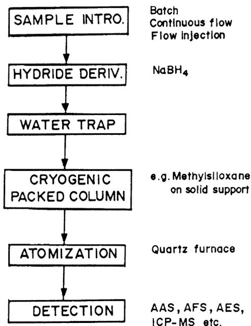
**Figure 5.** Schematic representation of hydride derivatization experiment, including trapping, atomization and detection. AAS, atomic absorption spectrometry; AFS, atomic fluorescence spectrometry; AES, atomic emission spectrometry; and ICP-MS, inductively coupled plasma-mass spectrometry.
